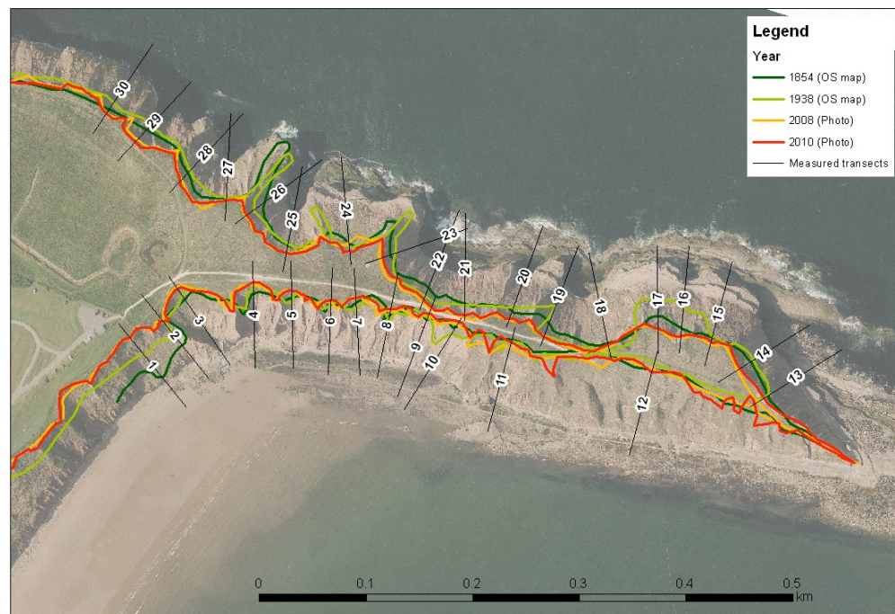
Figure 12. Location of measured transects and digitised coastlines used in the recession analysis
